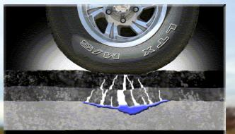
**Reduce it** Stop a major % of the cracks **Retard it Delay the reflection through an surface** treatment. **Control it** Install a seal so that the crack that reflect don't deteriorate the pavement.
