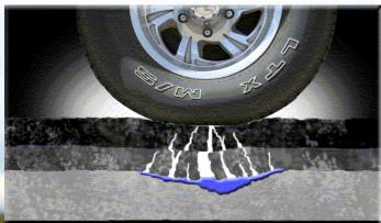
**Reduce it** Stop a major % of the cracks **Retard it Delay the reflection through a surface** treatment. **Control it** Install a seal so that the cracks that reflect, don't deteriorate the pavement.
